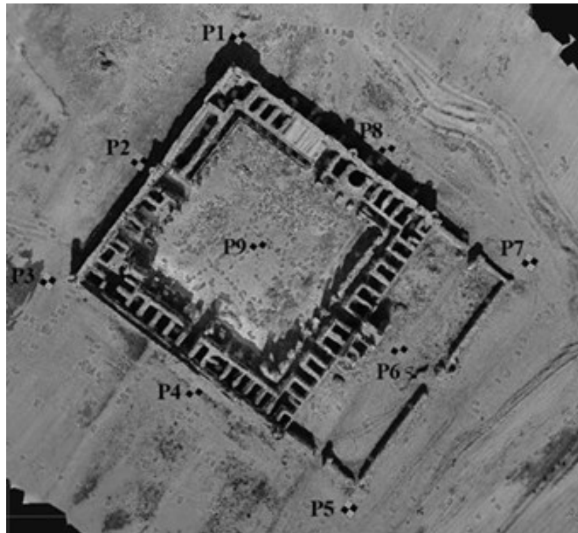
Figure 3. Approximate position of targets on the caravanserai's enclosure used by the Drone(Samadzadegan et al., 2023)
