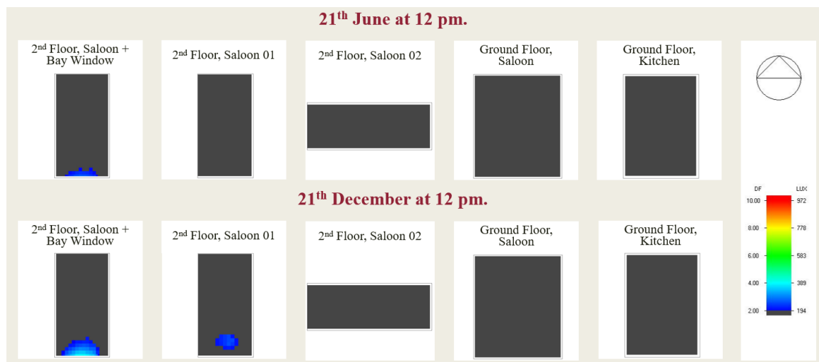
Figure 7: The daylighting performance of the case study building at 12 pm in 21 st June and 12 pm in 21 st December.
