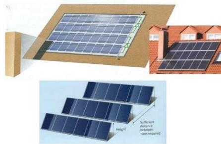
**Figure 7.** Shading effects from building fixtures, [16]
