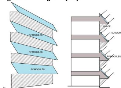
**Figure 4.** PV facade consisting of overhanging PV shade screens, [11]
