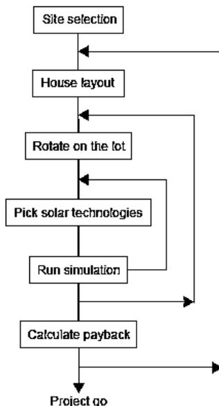
Figure5. Steps for solar construction, [22]
